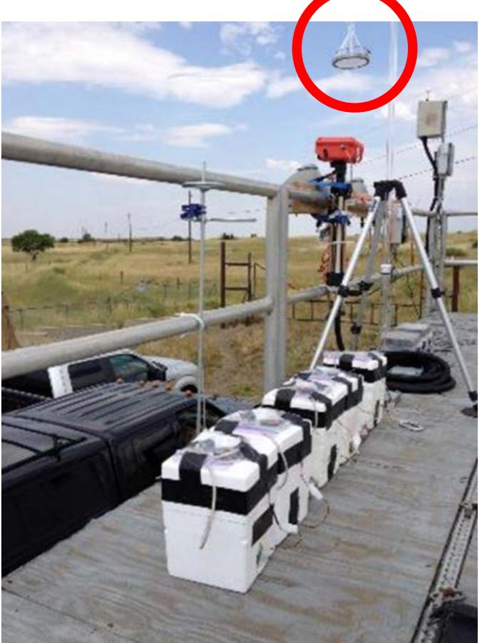
**Left:** Chemiluminescence cartoon and NO<sub>2</sub>-sonde schematic illustrating flows and key design features. **Middle:** D-AQ site map showing Golden; **Far right:** Five sondes placed on the EPA trailer roof close to the CAPS/CRDS inlet (red circle) for a side-by-side measurement at the Golden site.
