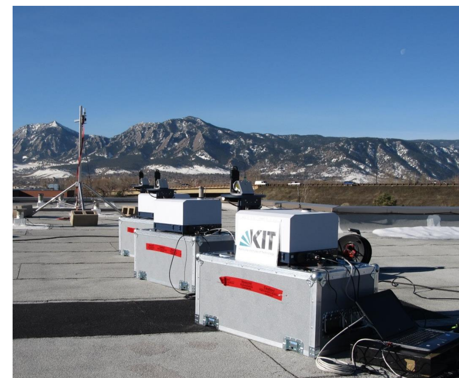
Figure 2: The EM27 FTS are easy to transport. For calibration upon arrival to Colorado they were co-located at NCAR.
