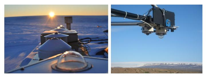
Two sets of three broadband radiometers, respectively for solar, infrared, and photosynthetic radiation, are installed on the roof (for the downward component) and on a mast (for the upward component) to measure the radiation budget at the surface and the surface albedo. Measurements of downwelling solar radiation were started by the Danish Meteorological Institute. ENEA is presently running the broadband radiation measurements carried out at THAOO.
