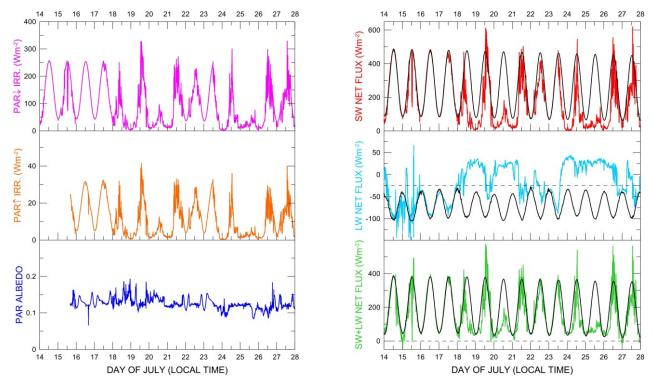
Left: time series of downward and upward PAR irradiance and derived surface albedo during the July 2016 SVAAP campaign; right: time series of the SW, LW, and total (SW+LW) surface net fluxes derived from measurements and for cloud-free conditions (black curves). The difference between measured and cloud-free curves is the radiative effect produced by clouds.
