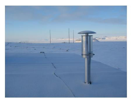
An aerosol sampler, collecting particulate matter of size < 10  $\mu$ m (PM10), was setup at Thule in 2010 by ENEA and University of Florence (Italy). The sampler collects particles on filters with a resolution of 48 hours. The filters are shipped to Florence and analyzed to determine aerosol load and particles' chemical composition.
