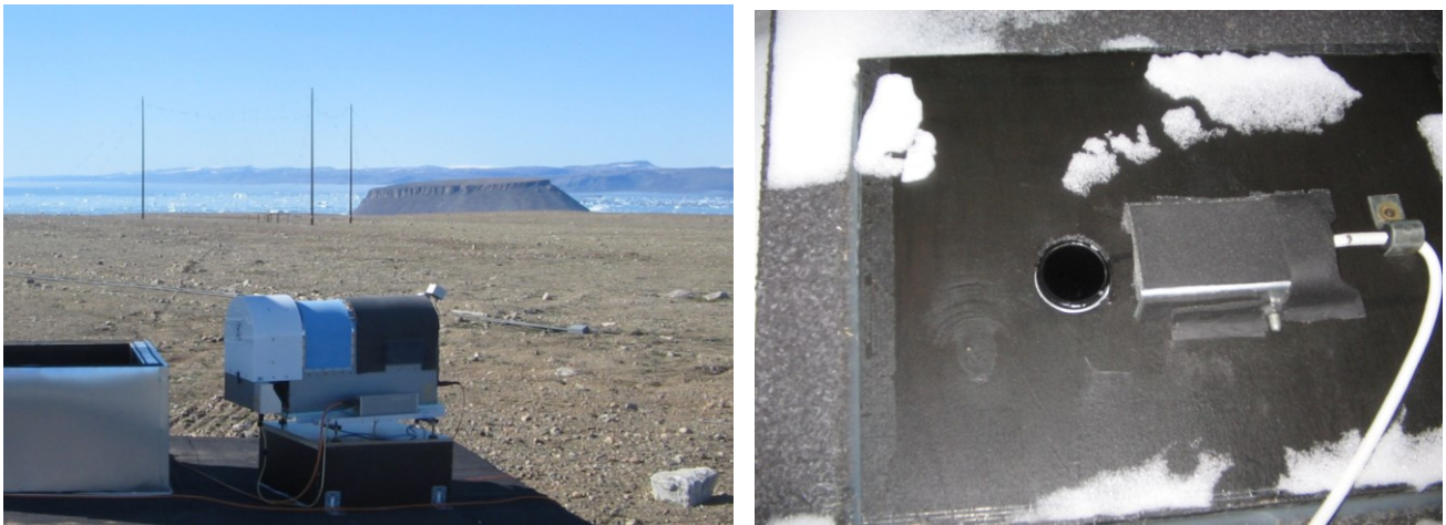
HATPRO microwave radiometer (left) and viewing port of the Heitronics pyrometer (right).
